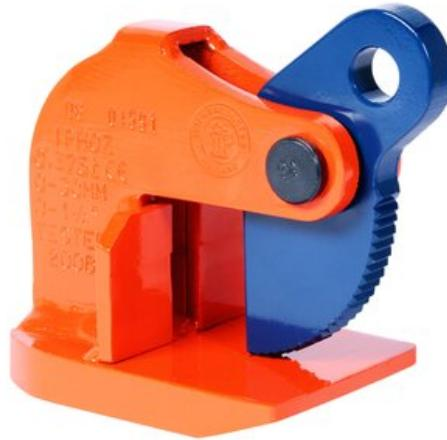
The IPHOZ horizontal lifting clamp is to be used for lifting and transferring, in the horizontal position, of thin sheet and other materials that will sag or bend when lifted. These clamps must be used in pairs or more.
