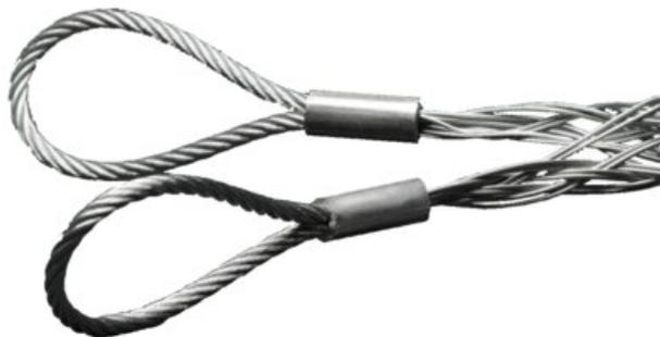
Stocking which can be opened with two impacted eyes for pulling-in of ropes or cables or check of hose. The grip can be placed anywhere along a cable, rope or hose and after that "sewed" together with a rope which are locked with wire rope clips.
