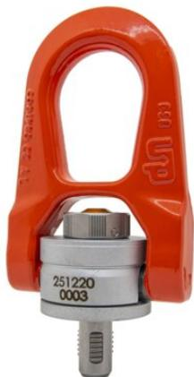
The QLR is a double swivel ring that allows particularly fast anchoring. At the push of a button, it can be fixed in the threaded hole in a matter of seconds. Its double swivel ensures a perfect alignment with the sling.
