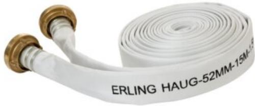
**General:** An all polyester single jacket product. It is of light weight and compact appx. half the weight of standard rubber lined jacket hose. It is highly resistance to most chemicals, petrol products, ozone and UV exposure, rot and mildew.
