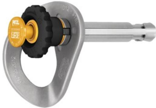
The COEUR PULSE 12 mm is a removable, high-quality stainless steel anchor that can be installed and removed for reuse very simply and rapidly without tools. The locking function limits the risk of accidental removal. The COEUR hanger can rotate once installed and when laterally loaded during use, allowing it to better align with the systems in place.
