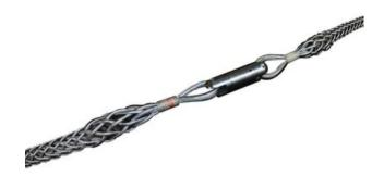
Back-2-back cable grip with inline swivel for installation of steel wire rope. The swivel helps prevent transfer of rotation from old to new steel wirerope.
