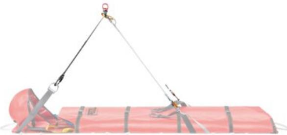
The STEF tilting device joins the three connection points of the NEST litter and allows it to be easily tilted according to the terrain. It has three Am'D TRIACT-LOCK connectors for automatic locking of the connection points, and a swivel for precise orientation of the litter.
